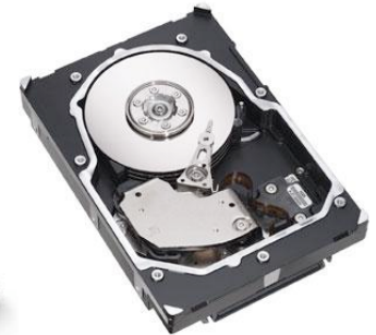
Hard Drives: 7W- 25W Temp Spec: 50C-60C
