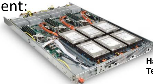
Rackable CloudRack C2 Temp Spec: 40C
